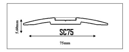
SC50 and SC75 Slim-Line Floor Cover Strips with secret fittings have been designed for smooth transition between different flooring surfaces. The initial design spec was to facilitate wheel chair access between rooms with vinyl flooring and carpeted corridors in a medical facility. The profiles have a smooth finish to reduce bacteria from forming. The cover strips are of a solid design for commercial installations, but would also suit domestic applications such as thresholds.
